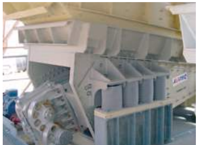
Compression spring support with gearing protection
