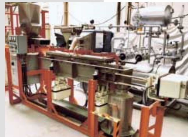
In the vibration fluidised bed, plastic granulate, for example, passes over a microsieve. Hot air dries precisely to the specified remaining moisture content. A close-loop control circuit regulates the speed of flow in dependence on the degree of drying, using simply voltage control on the drives
