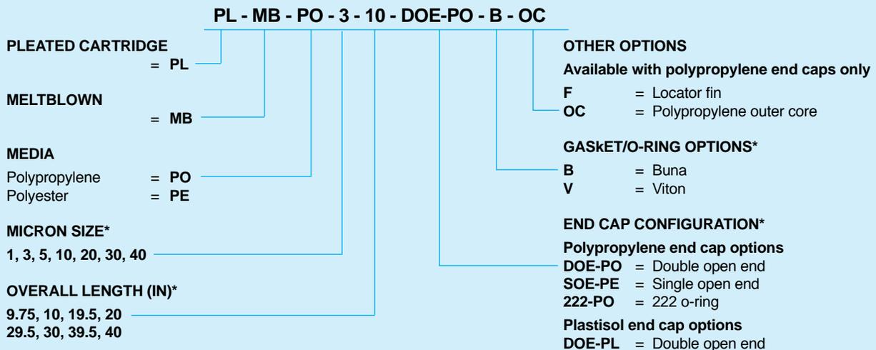
\*Other micron sizes, lengths, end cap configurations and gasket/o-ring options may be available
