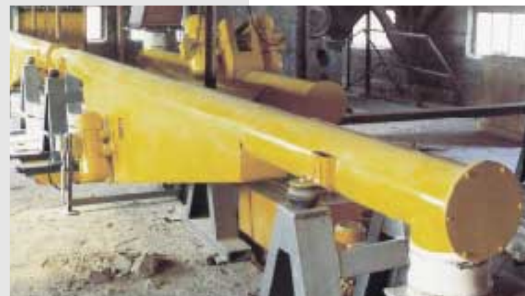
Enclosed conveying protects from unwanted contamination of the transported material and of the environment
