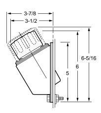
Where top surfaces are not available for locating a filler port, this unit mounts on vertical tank walls. The housing is tough, glass-reinforced nylon. It's only available with a 3-in. deep basket (and optional inner guard). The only other options are the 3-in. dipstick, the lockable cap, and powder coated cap.
